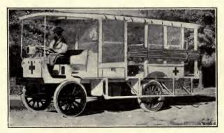
British ambulance, heavy type. Capable of carrying 8 sitting or 4 lying -down. Litters are carried on its sides. Also equipped with emergency dressings. Cool in hot weather; during rain side curtains can be lowered.
