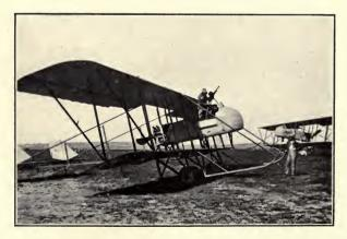
At the French aviation field, two miles from Belgrade. Eighty horsepower motor biplane. Capacity, two passengers. Plane has glass floor, carries five large bombs, five cans of flashettes, and other accessories. Aviator is cleaning and adjusting the Hotchkiss rapid-fire gun, preparatory to making a flight.
